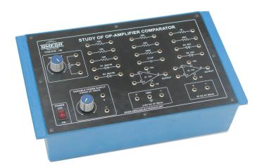
**OMEGA TYPE ETB-150** Experimental Training Board has been designed specifically for the study of OP-AMP Cooperator.
