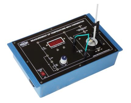
**OMEGA TYPE ETB-145** Experimental Training Board has been designed specifically for understanding the Temperature Measurement technique using a Thermistor. The board is absolutely self contained and requires no other apparatus.
