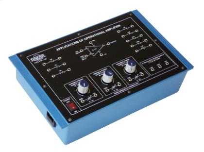
**OMEGA TYPE ETB-159** Experimental Training Board has been designed specifically for the study of basic Applications of operational Amplifier (OP-AMP) using IC-741.
