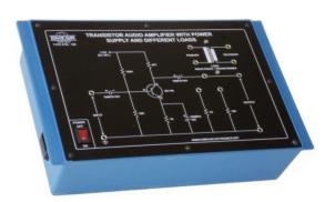
**OMEGA TYPE ETB-160** Experimental Training Board has been designed specifically for the study of single stage Transistor Audio Amplifier with three different loads.
