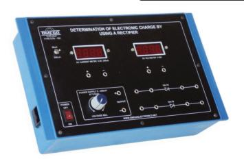
**OMEGA TYPE ETB-162** Experimental Training Board has been designed specifically for determination of electronic charge (e) by using rectifier equation in case of a point contact germanium rectifier. The board is absolutely self contained and requires no other apparatus.
