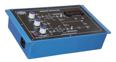
**OMEGA TYPE ETB-168** Experimental Training Board has been designed specifically for the study of Window Detector using OP-AMP ICs 741. This Training Board gives a better understanding of the detection of Input signal when lying between a specified range of voltages. The board is absolutely self contained and requires no other apparatus.
