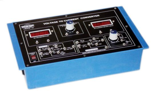
OMEGA TYPE ETB-169 Experimental Training Board has been designed specifically to study Voltage to Current Converter using OP-AMP ICs 741. This Training Board gives a deep understanding of the conversion of voltage into proportional current in both Inverting & Non-Inverting configurations. The board is absolutely self contained and requires no other apparatus.
