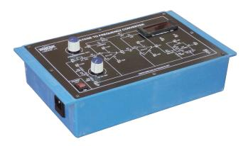
OMEGATYPE ETB-171 Experimental Training Board has been designed specifically for the study of Voltage to Frequency Converter using OP-AMP ICs 741. This Training Board gives a better understanding of the conversion of Input D.C. voltage into proportional output frequency.
