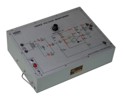
**OMEGA TYPE ETB-172** Experimental Training Board has been designed specifically for the study on Under Voltage Monitoring using OP-AMP IC 741. This Training Board gives a better understanding of the detection of input voltage when going below the specified range.
