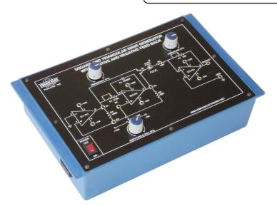
OMEGA TYPE ETB-165 Experimental Training Board has been designed specifically for the study of Square and Triangular Wave Generator with Positive and Negative Feedback using OP-AMP ICs 741. This Training Board is designed using Schmitt Trigger, Integrator and Inverting Amplifier to generate Square & Triangular waves using feedback principle. Also there are potentiometric controls for the change in Frequency, Amplitude and Duty cycle of waveforms.
