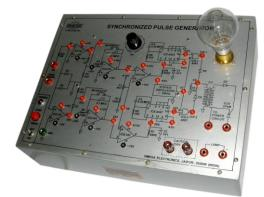
**OMEGA TYPE ETB-177** Experimental Training Board has been designed specifically for the study of Synchronized Pulse Generator. This Training Board gives a better understanding on the generation of Sync. pulses to trigger SCR in synchronism with the supply voltage using phase control principle.
