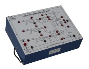
OMEGA TYPE ETB-178 Experimental Training Board has been designed specifically for the study of Phase Sequence Monitoring. This Training Board gives a better understanding to detect whether the incoming low voltage three phase signal is in proper phase or not.
