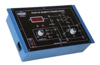
**OMEGA TYPE ETB-181** Experimental Training Board has been designed specifically for the study of Schmitt's Trigger Circuit based on IC-741. This Training Board is quite useful in studying the hysteresis associated with the schmitt trigger and the effect of feedback on threshold voltages.
