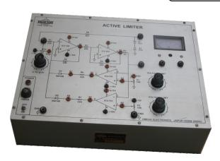
OMEGA TYPE ETB-173 Experimental Training Board has been designed specifically for the study of Active Limiter using OP-AMP ICs 741. This Training Board gives a better understanding of the principles of limiting of input voltage at output with specified limits of +ve & -ve voltages. The board is absolutely self contained and requires no other apparatus.
