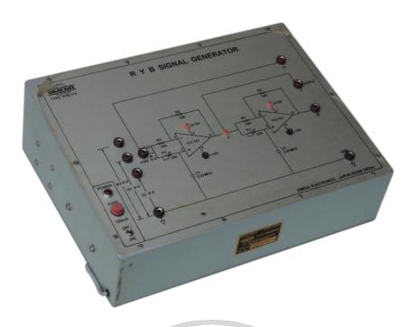
OMEGA TYPE ETB-174 Experimental Training Board has been designed specifically for the study of R Y B Signal Generator using OP-AMP ICs 741. This Training Board gives a better understanding of the generation of two additional sinusoidal signals from single phase with 120° phase shift using OP-AMPs to obtain virtual RYB sinusoidal signals.
