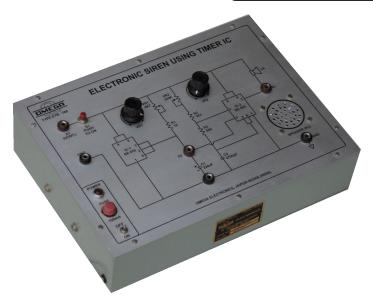
**OMEGA TYPE ETB-188** Experimental Training Board has been designed specifically for the study of Electronic Siren using Timer ICs. This training board gives a better understanding of timer IC application as a Astable Multivibrator & frequency modulation of timer O/P with the sawtooth voltage.
