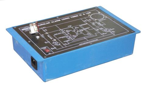
**OMEGA TYPE ETB-189** Experimental Training Board has been designed specifically to study the Burglar Alarm using Timer IC & LDR. This training board gives a better understanding of timer IC application as a Astable multivibrator.
