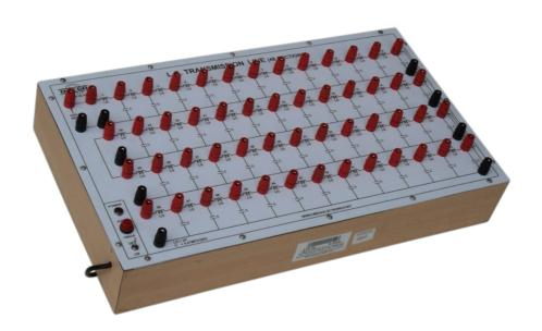
**OMEGA TYPE ETB-192** Experimental Training Board has been designed specifically to the study of L-C Transmission Line (48 sections).
