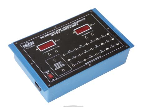
OMEGA TYPE ETB-183 Training Board has been designed specifically to determine the Internal Resistance of a D.C. source by matching a load for maximum power transfer. The board is absolutely self contained and requires no other apparatus.
