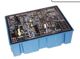
**OMEGA TYPE ETB-185** Experimental Training Board has been designed specifically for the study of Switching Mode Power Supply (SMPS) for computer. Now a days Switching Mode Power Supplies are extensively used in various electronic instruments and computers.
