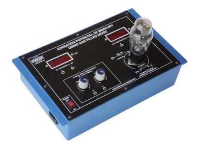
**OMEGA TYPE ETB-197** Experimental Training Board has been designed specifically to find the ionisation potential of mercury using gas filled diode. The board is absolutely self contained and requires no other apparatus.
