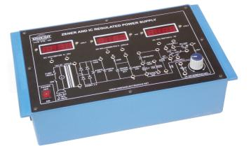
**OMEGA TYPE ETB-199** Experimental Training Board has been designed specifically for the study of zener regulated and IC regulated power supply. This training board is absolutely self contained and requires no other apparatus.
