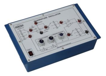
**OMEGA TYPE ETB-194** Experimental Training board has been designed specifically to study of quadrature oscillator. It produces sine wave and cosine wave that are in out of phase by 90°.
