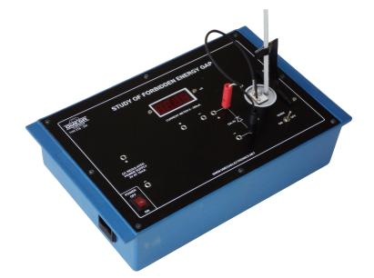
**OMEGA TYPE ETB-204** Experimental Training Board has been designed specifically to study the Forbidden Energy Gap in Semiconductor Diode. The board is absolutely self contained and requires no other apparatus. Practical experience on this board carries great educative value for Science and Engineering Students.
