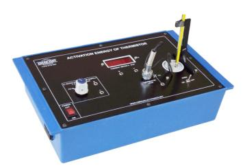
**OMEGA TYPE ETB-205** Experimental Training Board has been designed specifically to determine the activation energy of a thermistor and to determine the material constant of the thermistor material.
